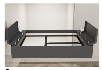
2 Attach the side brackets to the frame using 3x2 screws. Use hole 1, 2 and 4.
